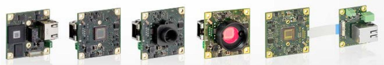
**GigE uEye LE board-level industrial camera: Compact CMOS single-board camera with excellent image quality and many additional features**
